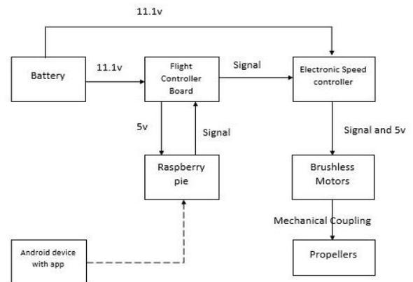
Fig 7: Block Diagram
