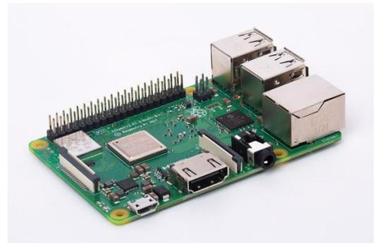
Fig 1: Raspberry Pi-3B plus model
